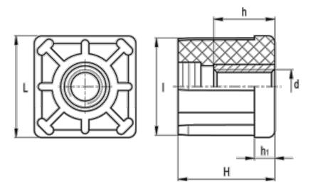
$\begin{array}{lll} d & = M16 \\ h & = 15 \\ H & = 45 \\ h1 & = 10 \\ Internal tube size = 44.0 \\ I & = 44.0 \\ L & = 50 \\ \end{array}$
